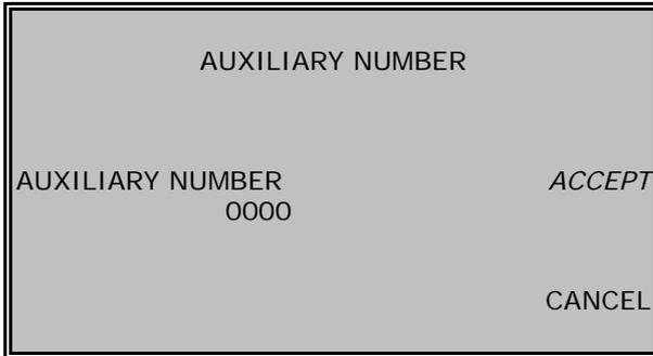
Use the keyboard to enter the Auxiliary number. These numbers can be changed individually by pressing **↑** or **↓** to change values from 0 to 9; press **→** or **←** to move the cursor right or left, respectively.
