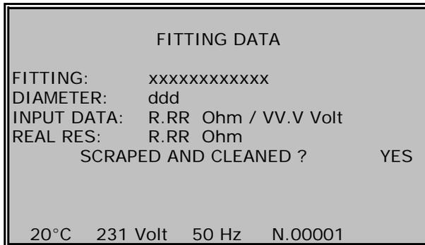
The fitting description, size and coded resistance will be on the screen only in the case of bar-code system has been used. The REAL RES corresponds to the value of the resistance read on the fitting, whereas the INPUT DATA corresponds to the resistance and voltage values provided by the bar-code.
