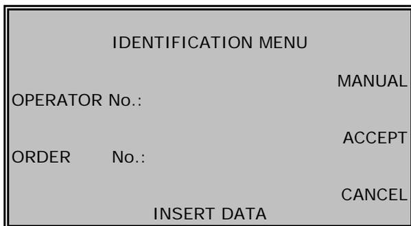
These identifications are compulsory. Proceed to enter the operator's ID\* (via barcode) and job order No. (via barcode or manually, either). Completed the introduction, ACCEPT will be displayed. Press it to continue.
