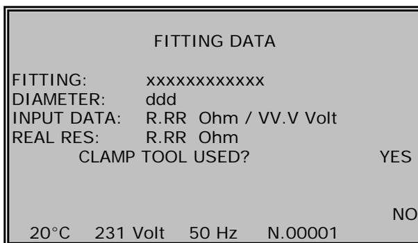
Press YES or NOT according the fitting installation used.
