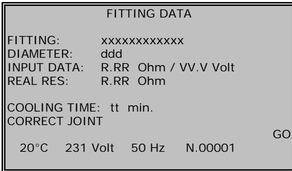
If the electrofusion cycle is completed satisfactorily, the message "CORRECT JOINT" will be displayed, along with the perceptive cooling time provided that it has been given by the fitting's manufacturer. See NOTE.
