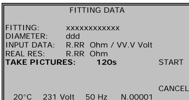
**NOTE:** not be fixed the LED *status* of the BlueBox, the message RUN APP BLUEBOX will appear. See point 1 of 2.3.3 **Run the application.** Once showed the message TAKE PICTURES, it will begin the countdown of 120 seconds to carry out the necessary photos (minimum 1, maximum 4).
